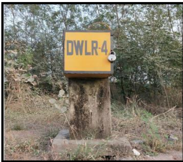
Photo 5 & 6: Showing Piezometric Well installed at different locations within Mines Area
