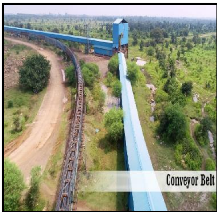
Photo 12: Showing Covered Conveyor Belt on the Right & Pipe Conveyor Belt on the Left
