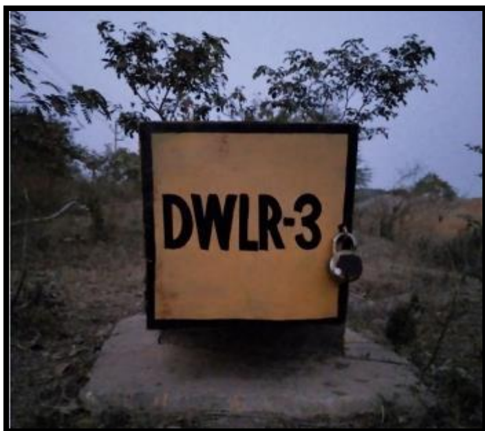
Photo 5 & 6: Showing Piezometric Well installed at different locations within Mines Area
